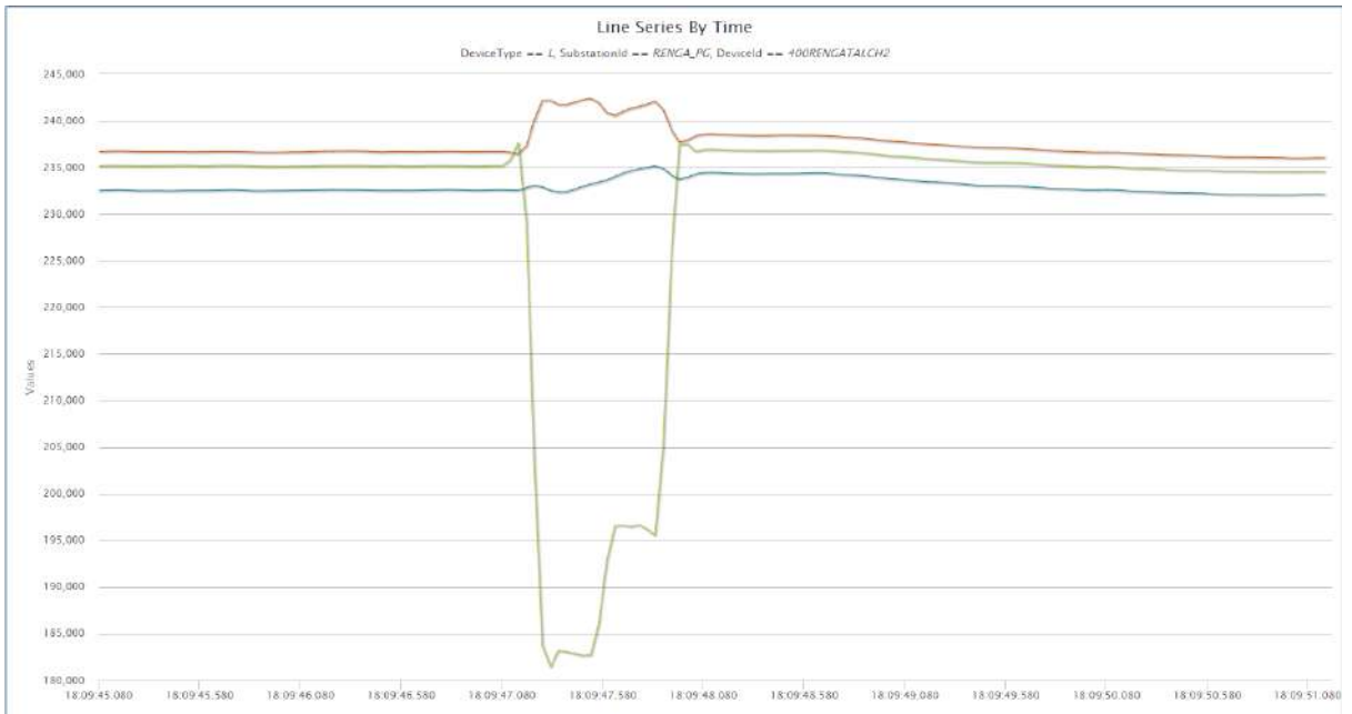
Figure 2: PMU Voltage snapshot of 220 kV Regali-Talcher-2
