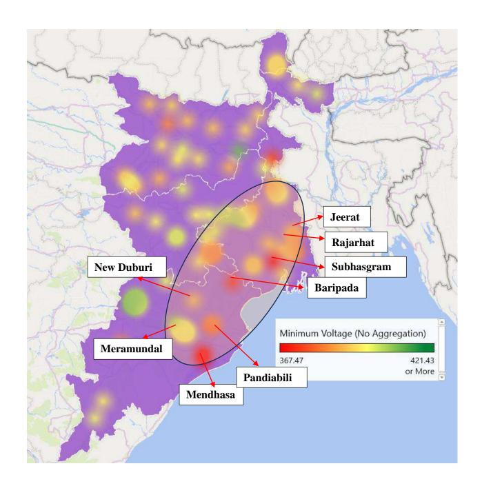
From the above heat map of voltage, it is observed low voltage issues observed in the southwestern part of the Eastern region due to mainly increased space cooling load with the increase of urbanization in this area.
