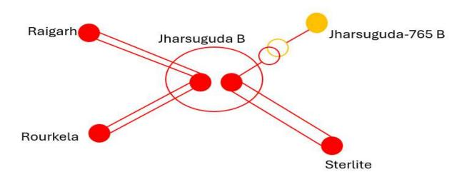
Post implementation of this scheme, a total 200MW Talcher generation backing down withdrawn. Parallelly the loading of 400 kV Jharsuguda – Rourkela 1 & 2 was reduced significantly.
