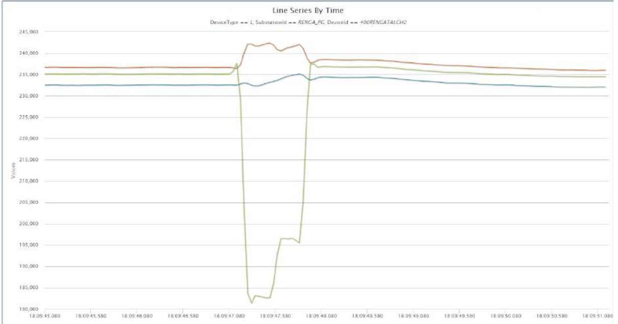
Figure 2: PMU Voltage snapshot of 220 kV Rengali-Talcher-2
