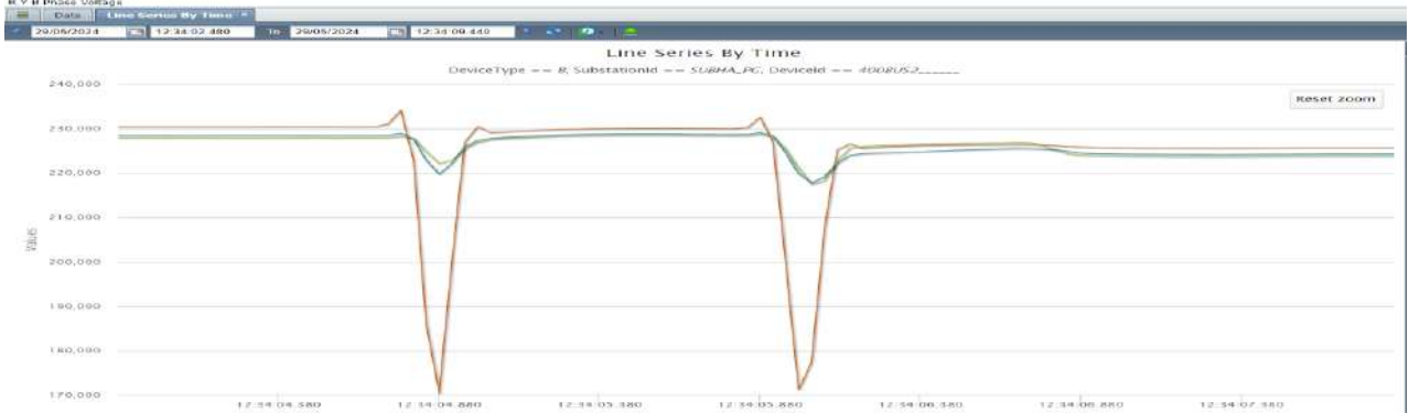
Figure 2: PMU Voltage snapshot of 400 kV Subhasgram S/S
