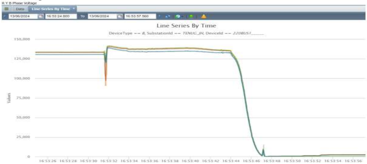
Figure 2: PMU Voltage snapshot of 400/220 kV Tenughat S/S
