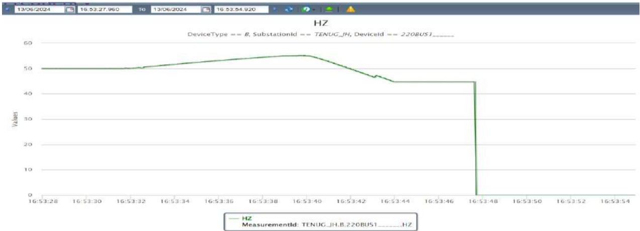
Figure 3: PMU Frequency snapshot of 400/220 kV Tenughat S/s
