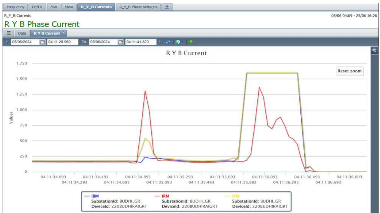
PMU Current snapshot of 220 kV Budhipadar-Raigarh
