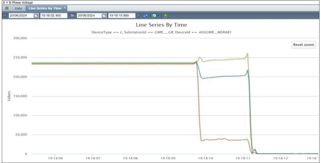
Fig4: -PMU Voltage plot of 400 kV GMR Meramundali – B
