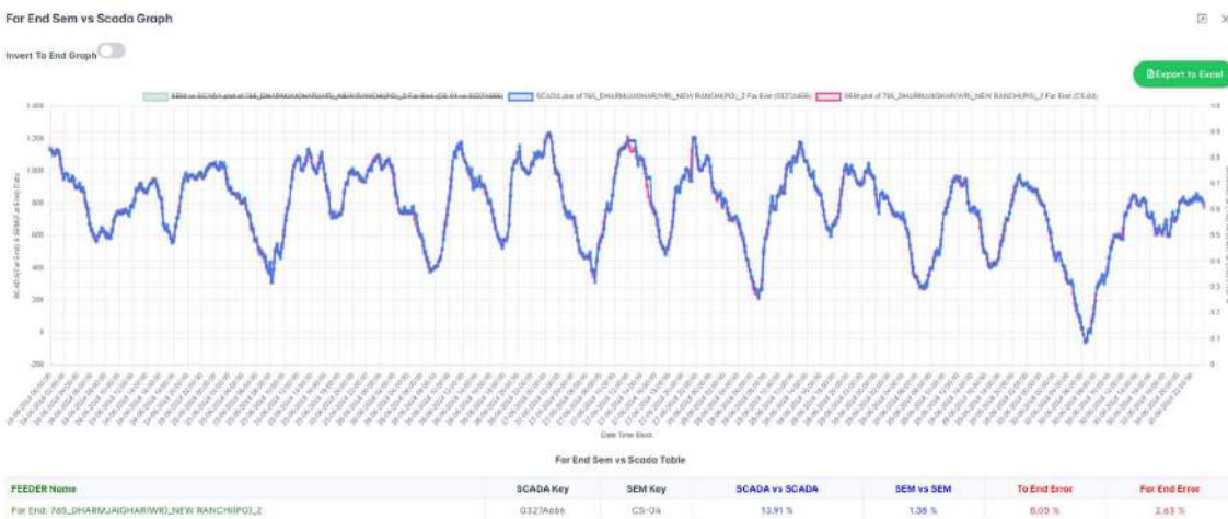
Plot: SEM vs SCADA data comparison at Dharamjaigarh End
