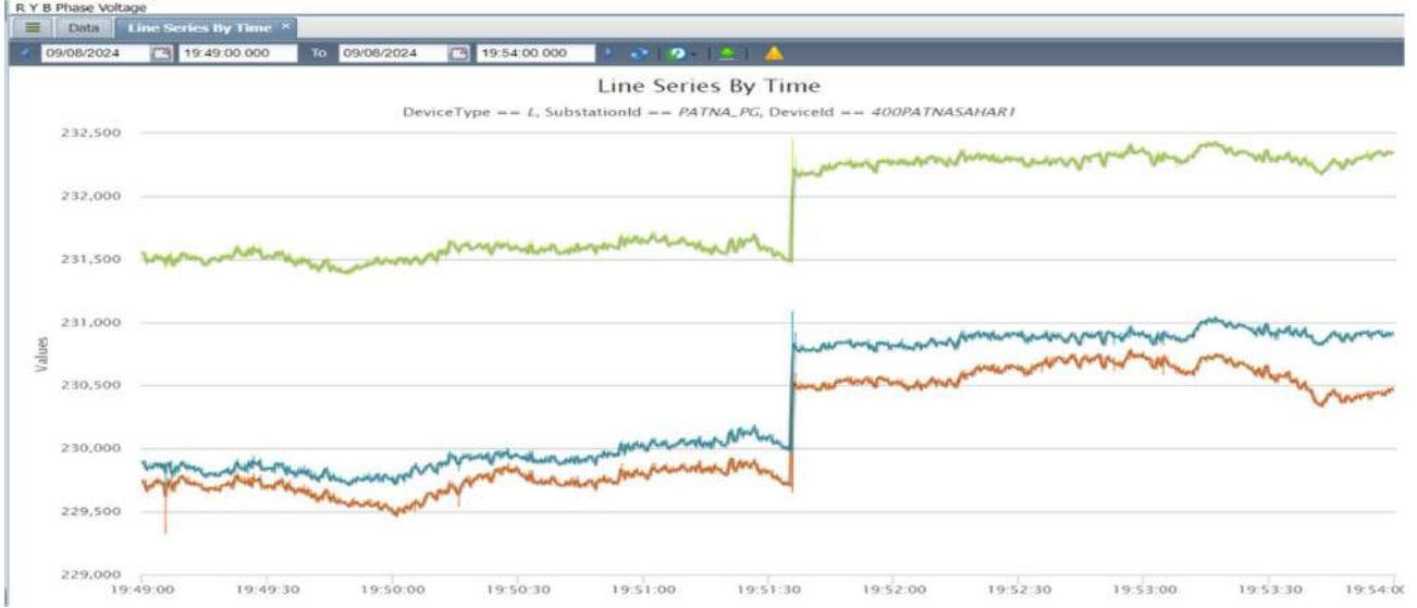
Figure 2: PMU Voltage snapshot of 400/220 kV Patna S/S
