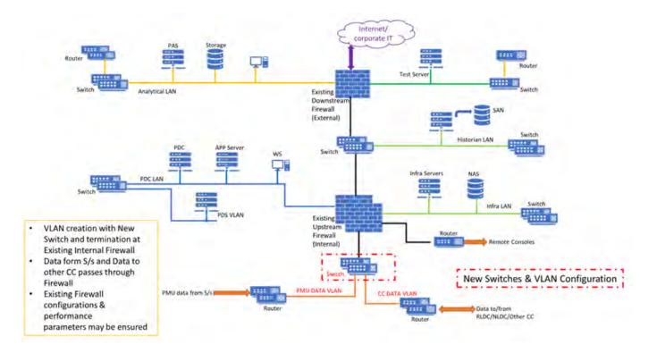
The PMU data is proposed to be routed through existing internal firewalls in the existing URTDSM system.
