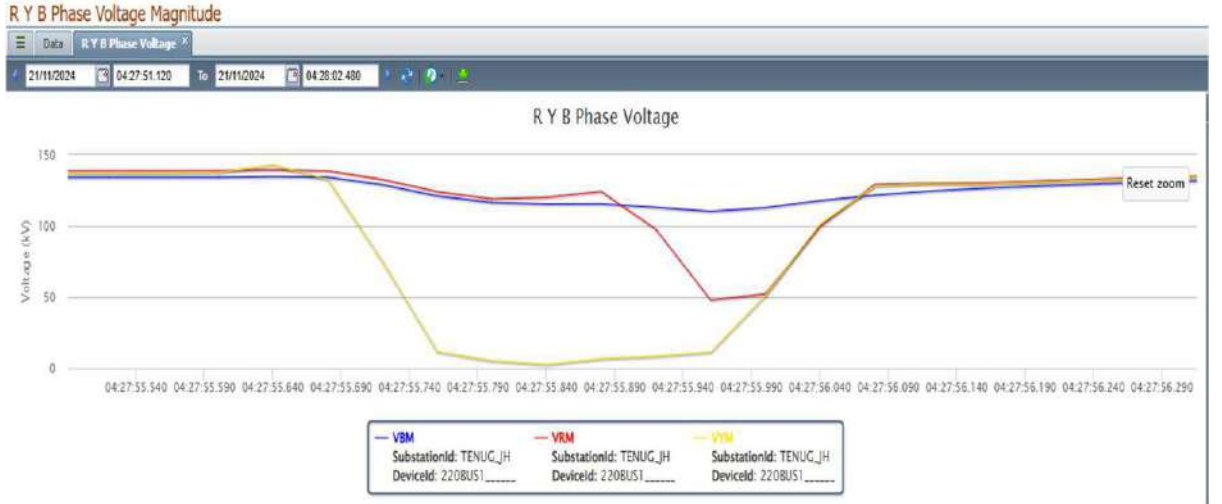
Figure 2: PMU of Bus voltage at Tenughat
