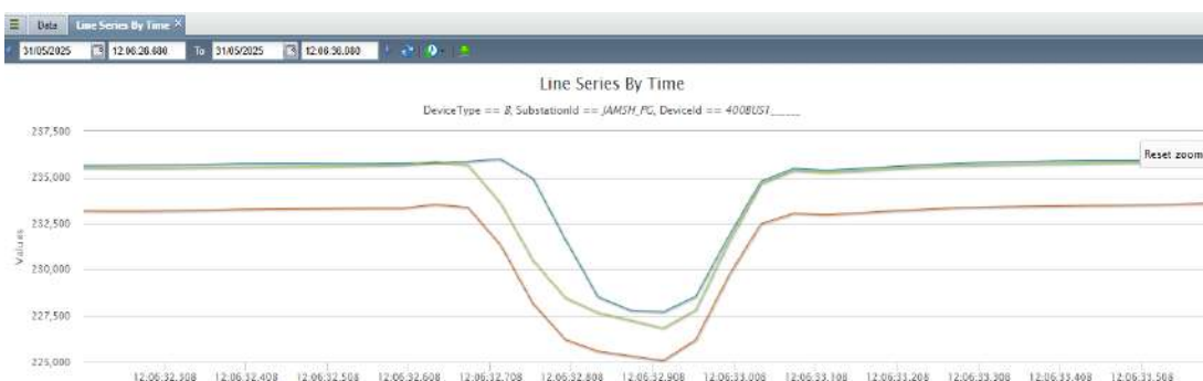
Figure 2: Fault clearing as seen in PMU
