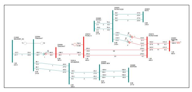
With high demand of Jharkhand and high injection from WR towards ER, single 400/220kV ICT at Tenughat may get loaded beyond 200 MW.
