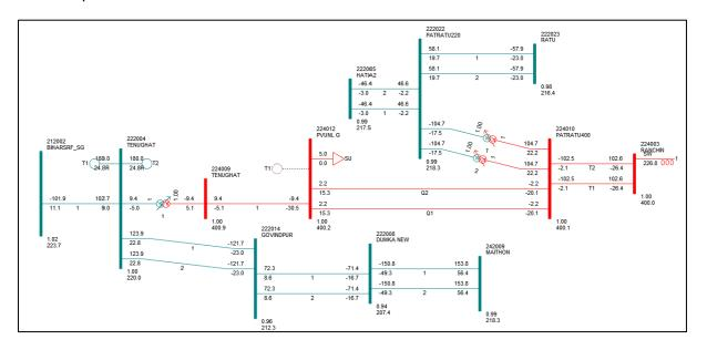
With both units of Tenughat in service, 9 MW is going from Tenughat to PVUNL via 250 MVA ICT at Tenguhat.
