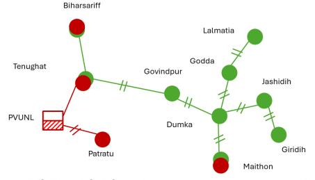
After discussion, JUSNL and SLDC Jharkhand decided that the 400 kV Patratu—Tenughat link shall be kept in continuous service to enhance the reliability of the Jharkhand power system. It was opined by the SLDC Jharkhand that this line significantly helping the state system by relieving constraints on the 220 kV Maithon—Dumka D/C and enabling the Dumka—Govindpur loop to remain in service under varying Tenughat unit availability, including
