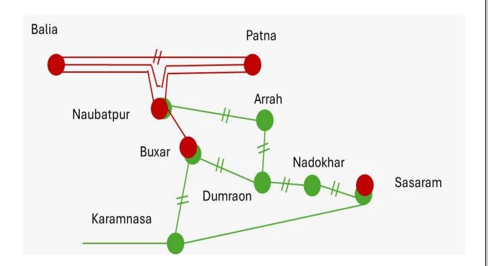
In the 54th TCC/ERPC held on 23–24 June 2025 at Chennai, Bihar confirmed readiness of intra-state system for injection of 1×660 MW Buxar TPS through existing interim arrangement of 400 kV Naubatpur–Buxar line with Bihar's 220 kV system.
