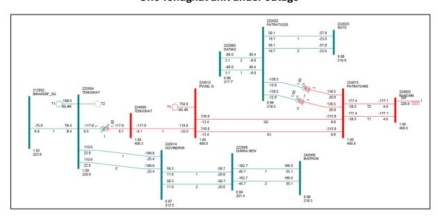
With full generation of PVUNL and only one unit of Tenughat in service, 118 MW is coming from PVUNL to Tenughat via 250 MVA ICT at Tenguhat.
