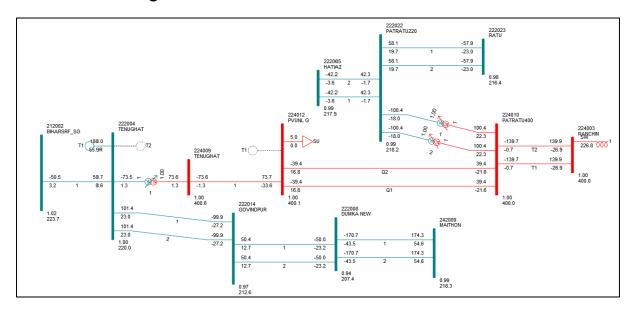
With one unit of Tenughat in service, 74 MW is coming from PVUNL to Tenughat via 250 MVA ICT at Tenguhat.
