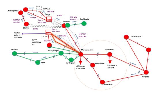
The emergency was managed through backing down of 600 MW generation at Talcher NTPC. At 23:41 hrs, 400 kV OPGC–Lapanga D/C was revived after isolating the faulty Tie Bay, stabilizing the system.
